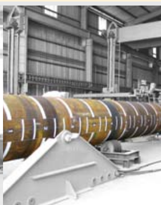
Completed leg or pile
