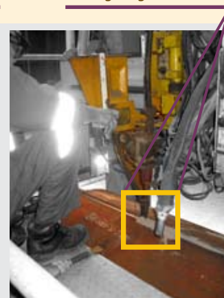
Welding long seam in cans
